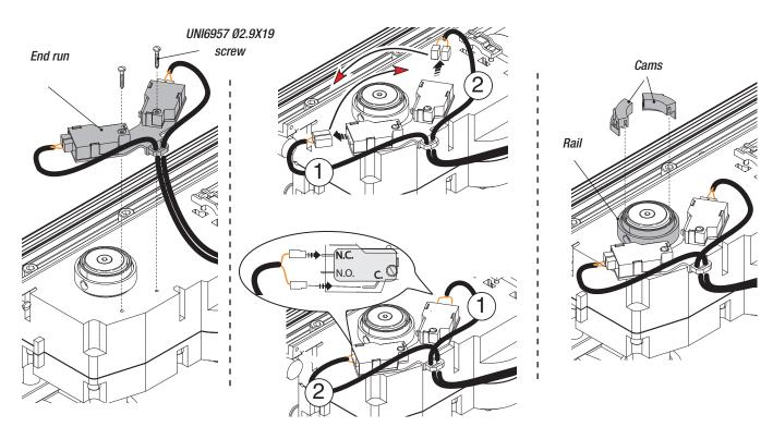
Close the leaf fully and turn the cam clockwise until the closing microswitch is activated. Secure the cam with the screws.
