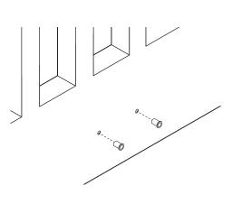
Position and secure the brackets as shown in the drawing.
