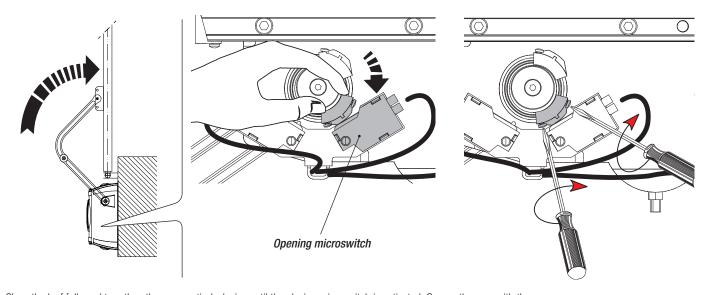
${\it Close the leaf fully and turn the other cam anti-clockwise until the closing microswitch is activated. Secure the cam with the screws.}$
