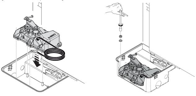
Lubricate the transmission lever.
